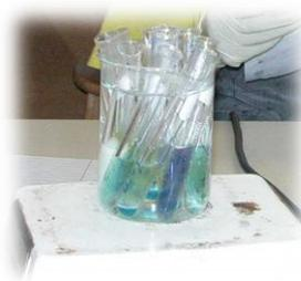
When heated, Benedict's solution will change color from blue to yellow, orange, or red in the presence of a simple sugar/ monosaccharide (reducing sugar). \*The green color represents a non-reducing sugar and needs to be tested using an additional method.
